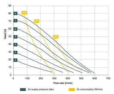
$^{\ast}$  The curves and performances refer to pumps with immersed suction and open delivery outlet with water at 20 °C and vary according to the composition materials.
