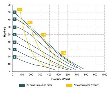
\* The curves and performances refer to pumps with immersed suction and open delivery outlet with water at 20  $^{\circ}\text{C}$  and vary according to the composition materials.
