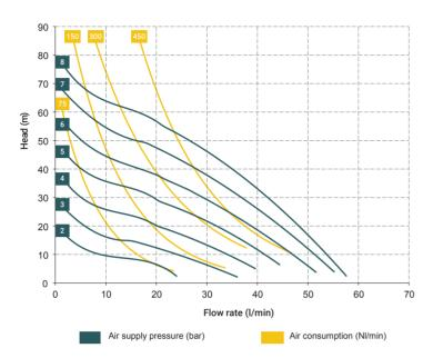
st The curves and performances refer to pumps with immersed suction and open delivery outlet with water at 20 °C and vary according to the composition materials.
